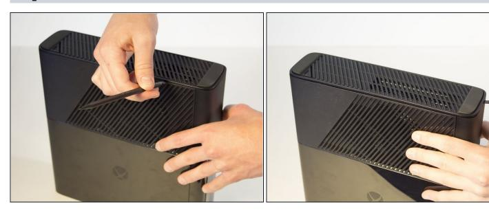
• Slide the spudger along the crevice to separate the grated face and the top body.
