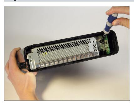
Remove the 11 mm screw left of the green wifi-card using the T9 Torx screw bit.
