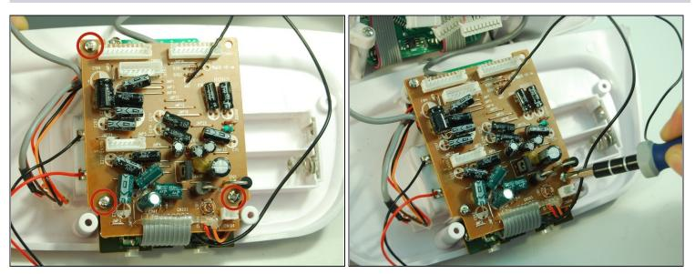
• Use the Phillips #1 Screwdriver to remove the three 8 mm screws holding the motherboard in place.
