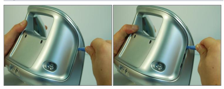
• To remove the back panel, use the plastic opening tool and gently work around the outline of the panel. The outline wraps around the sides and can be spotted at the top back of the device.
