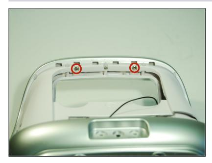
• Use a Phillips #1 screwdriver and remove the two vertical 8 mm screws from the top.
