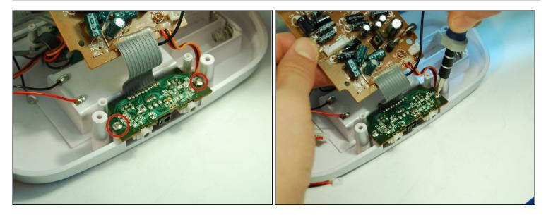
• Detach the smaller green audio port daughterboard by removing the two 8 mm screws with a Phillips #1 screwdriver.
