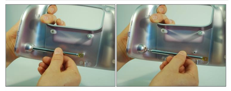
• If desired, the antenna can now be removed by pulling **inwards** and horizontal to the panel bottom.
