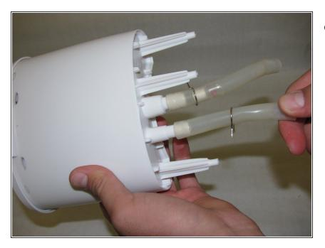
Carefully pull the silicon tubing off of the plastic tubing on the upper assembly.
