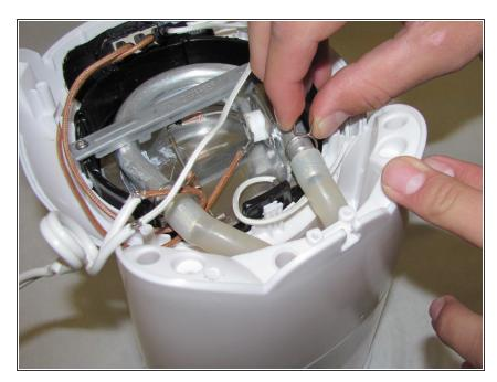
• Using your fingers, gently pinch and detach the two metal clips that secure the silicone tubing to the metal tubing on the TF6.
