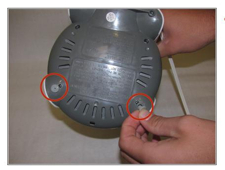
Facing the bottom of the TF6, carefully pull the two rubber feet out with your hands.
