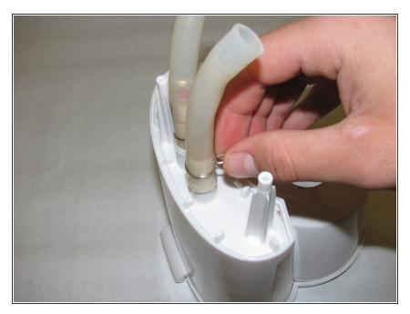
Using your fingers, gently pinch and detach the two metal clips that secure the silicone tubing to the plastic tubes on the upper assembly.
