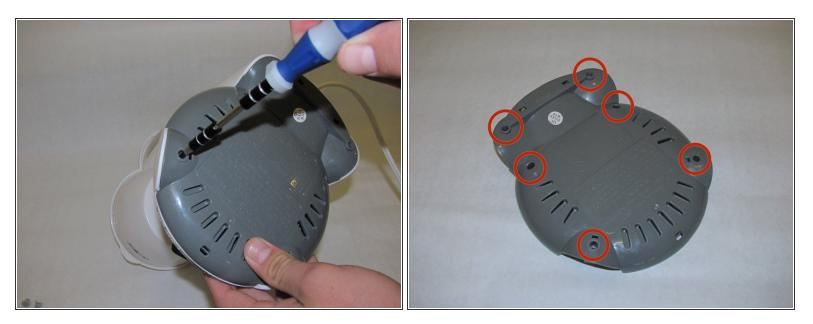
Using a Phillips #1 screwdriver, remove the six 11mm Phillips screws that are holding the bottom cover in place.
