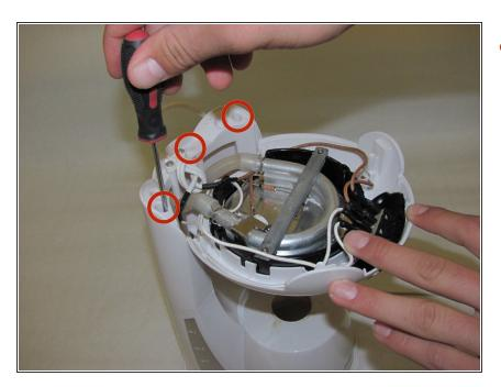
• Using a Phillips #1 screwdriver, remove the three 13mm Phillips screws that hold the lower and upper assemblies together.
