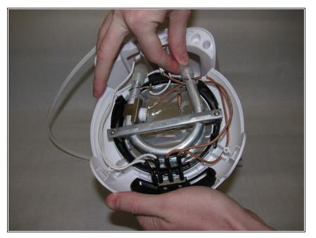
• Carefully pull the silicon tubing off of the metal tubing.
