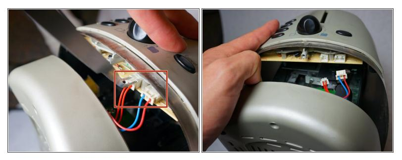
Disconnect the cable clips from the circuit board using the tweezers to free the outer metal shell from the plastic base.
