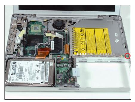
Remove the single Phillips screw securing the hall effect sensor board to the optical drive.
