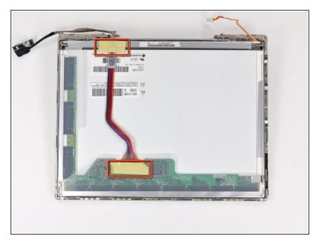
• Remove the two pieces of tape covering the display data cable.
