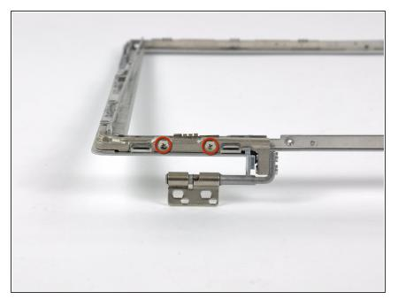
Remove the two 5.5 mm Phillips screws securing the right clutch cover to the front display bezel.
