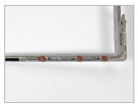
Remove the three 3.0 mm Phillips screws securing the right clutch cover to the front display bezel.
