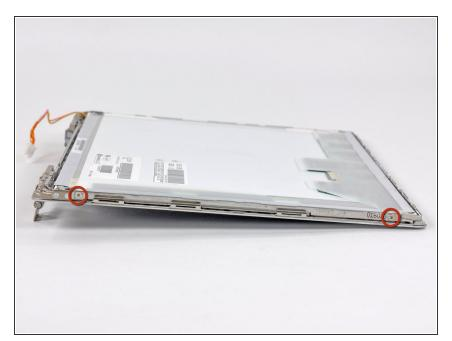
Remove the two 3.0 mm Phillips screws securing the LCD to the left side of the front display bezel.
