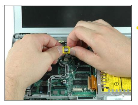
Lift up middle speaker cable from the lower left corner of the fan, and disconnect the two sections of the cable.
