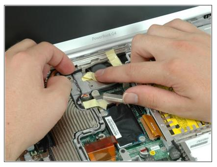
• Peel back the yellow tape securing the inverter cable near the fan.
