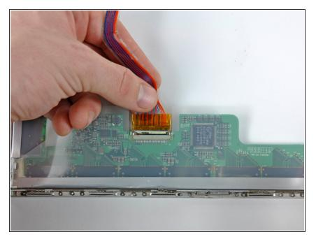
Pull the display data cable connector away from its socket to disconnect it from the LCD.
