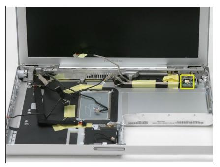
• Disconnect the multicolor connector by sliding it to the left.
