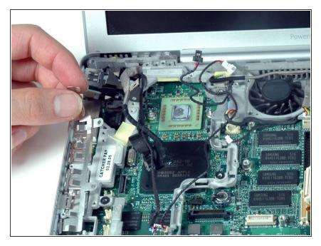
• Lift up and remove the silver EMI fingers located above the ports on the left side of the computer.
