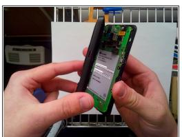
Now that the screws are removed, grab a spudger tool or a thick guitar pick. Start at the volume rocker and work your way around the phone by carefully pulling back the frame.
