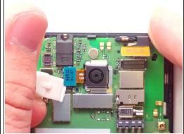
We're inside! At this step, there are 3 ribbon cables we need to disconnect to continue. Carefully pull these ribbon connections up.
