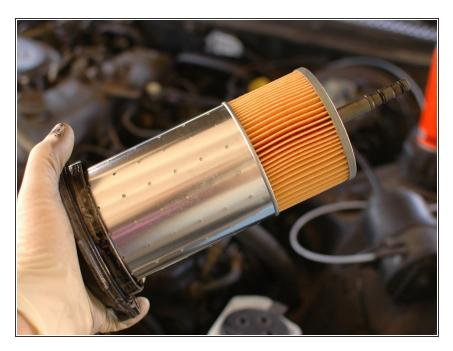
Install the new filter on the housing lid shaft. Then insert the filter in to the housing and snug the lid down with the two nuts you removed in step 5.
