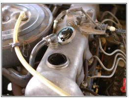
To start, remove the oil cap. This will allow the oil to drain out of the engine faster.
