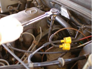
Next, loosen the two nuts that hold the lid on the oil filter housing. They take a 13mm socket just like the drain plug.
