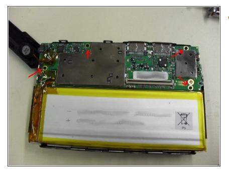
Under the screen you will find the top of the motherboard. There are four screws holding the motherboard and the hard drive together. After you remove those, the back of the device will come off.
