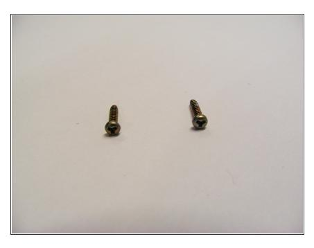
The Two screws at the top of the back panel can be unscrewed using a Y-triwing screwdriver.
