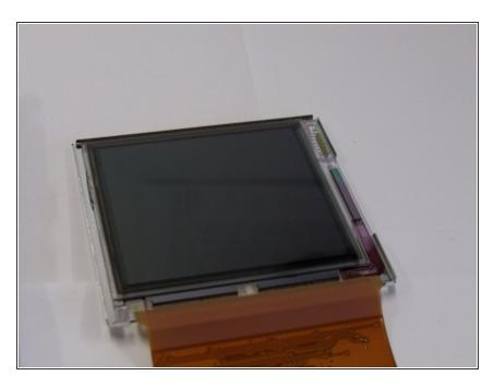
Peel of the protective film on the LCD screen and remove the LCD screen from the casing.
