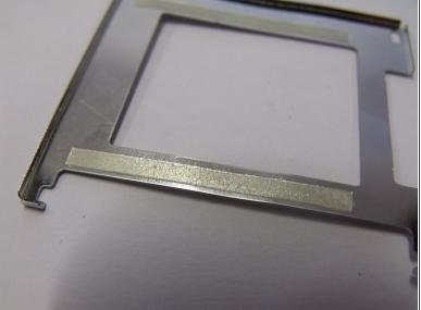
The metal on the screen can be pulled off by getting under it with your fingers this is stuck with a tape.
