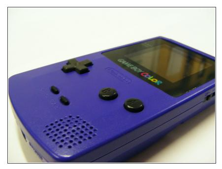
Take the Game boy and notice the way that it has been injection molded using two tools on the injection molder. The first thing to do is to separate these parts.
