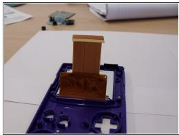
Once the foam is off you can pull the main connection of the screen out this is the brown part of plastic sheeting it simply slides out.
