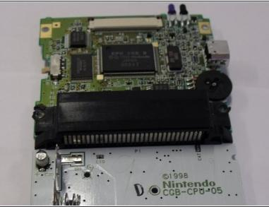
To remove the main board just remove the 4 screws in the back doing this will mean you can take the board out of the abs plastic sections.
