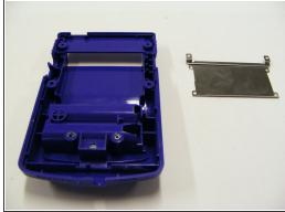
The metal cassette holder on the back plastic panel can be removed by simply using a small screw driver in all four corners this should mean it pops off.
