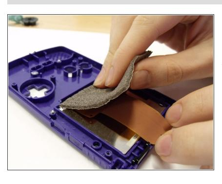
You can simply pull the foam off the back of the screen pulling off the glue try not to tear the foam this makes things easier later.
