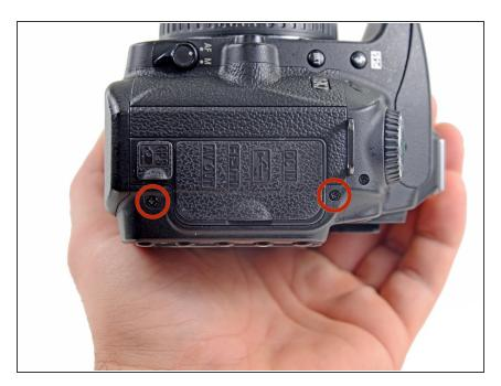
Remove the two 6.4mm Phillips screws on the left side of the camera, near the I/O ports.
