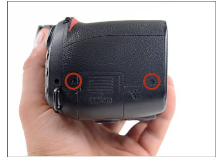
Remove the two 6.4mm Phillips screws on the right side of the camera, near the SD card slot.
