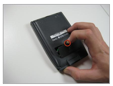
Push down and lift up the battery cover to remove it.
