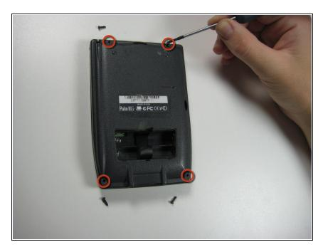
Using a Phillips #00 screwdriver, remove the four screws that hold the back cover in place.
