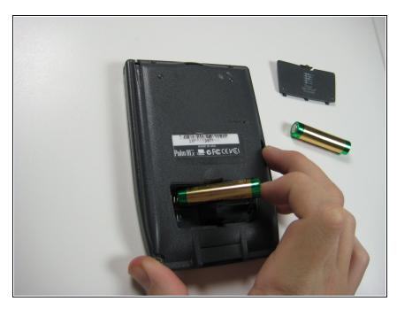
• Remove the old batteries one at a time.
