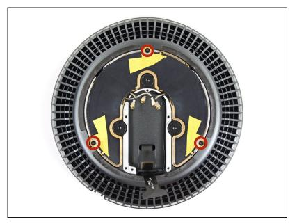
Remove the three 3.7 mm T4 screws securing the antenna array to the fan assembly.
