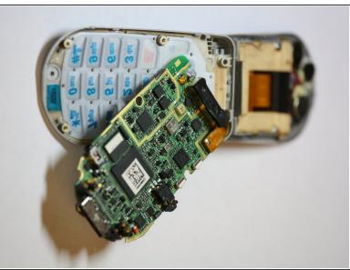
The logic board is only held on with 4 tabs and a data cable in the top right. Simply pry from one side using a screwdriver, popping out the board, before lifting the display data cable.
