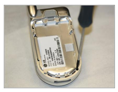
Remove the 4 small screws from the back panel, under the battery, using 00 Phillips-head.
