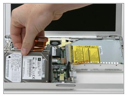
Use the orange cable to pull the hard drive up, then pull it and the hard drive bracket out of the computer.
