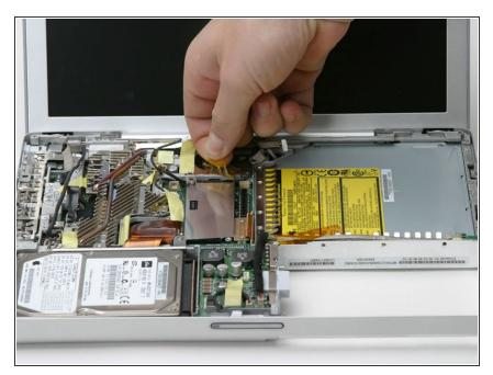
• Remove the orange tape on the trackpad side of the fan to free the fan cable.
