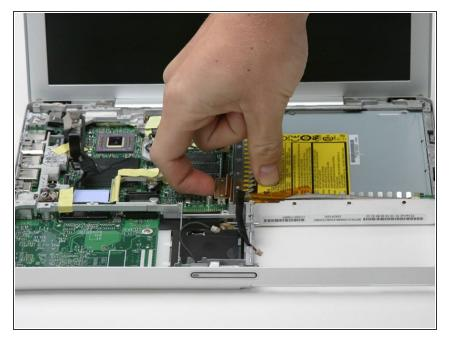
• Disconnect the orange optical drive cable from the logic board.
