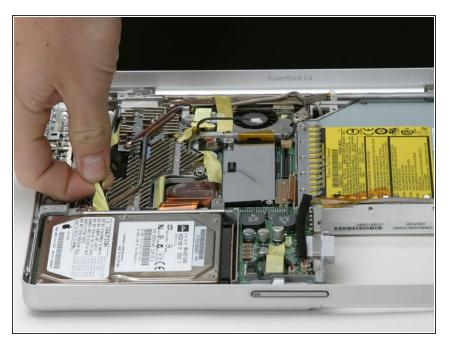
Remove the yellow tape to free the cable from the left side of the heat sink.
