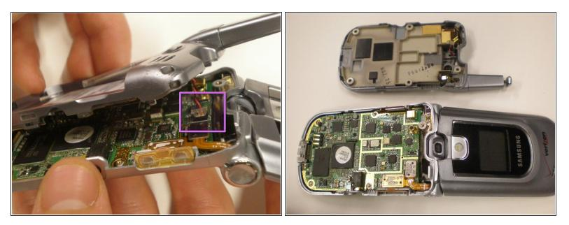
Gently unplug the external speaker wire from the logic board. After the wire is unplugged the back cover should come off easily.
