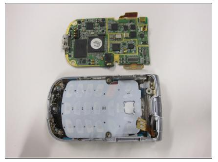
• Once logic board is removed, the back of the Keypad will be visible.
