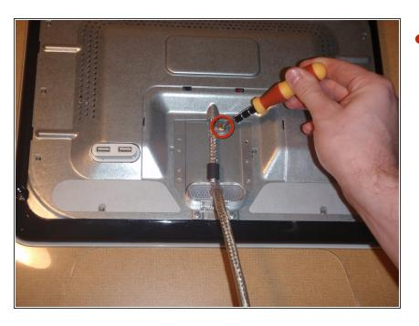
Remove the cable hold-down with #2 phillips head screwdriver.
