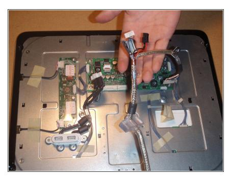
Finally, the main cable can be replaced by pulling the old cable away and repeating the previous steps in reverse with a new, working main cable.
