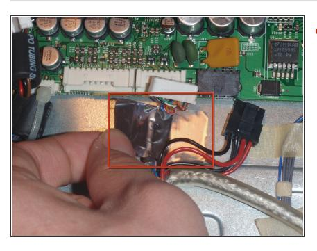
Remove tape holding down the white connector to the LCD main board.
