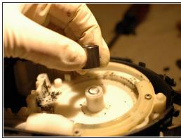
Lift the metal gear bushing up and off of the housing and set it aside.
