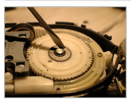
Use a metal spudger or flat blade screwdriver to remove the c-clip holding the gears to the bushing and shaft.
