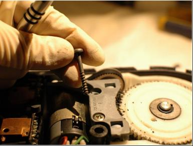
Continue disassembly by unscrewing the two Phillips screws holding the electric motor in place.
