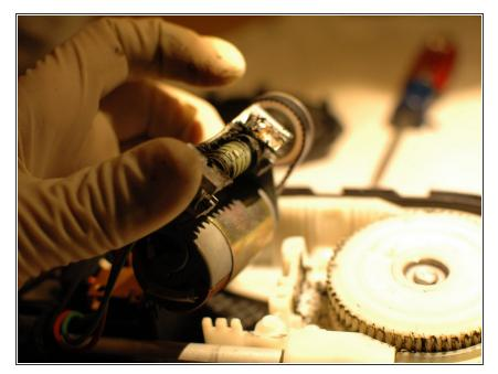
As the gears begin to lift, the electric motor will likely pop loose. It can be rested off to the side; it is wired to the control board so it cannot be removed fully at this time.
