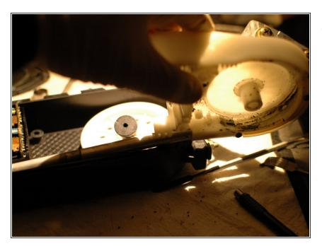
Now you can remove the gear and cable housing. It seems to work best to rotate the housing up and in the direction of the antenna shaft opening before angling it up and pulling it out of the motor body.
