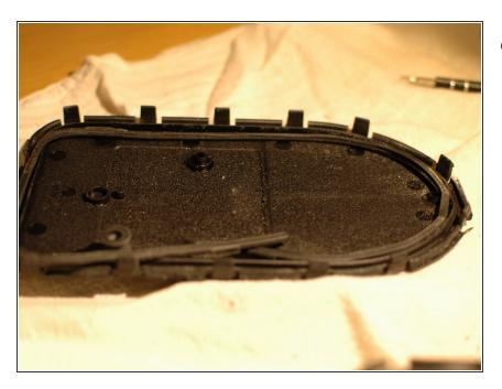
Make note of the rubber seal that goes around the body of the motor in a channel, sealing the cover to the body. If this seal is old a dry rotted it will need to be replaced, or a proper liquid sealant will need to be used in its place, if the motor is being reused.
