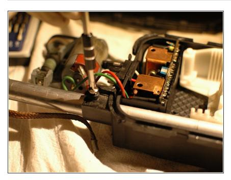
Unscrew the Phillips head screw that helps hold the antenna shaft to the body.
