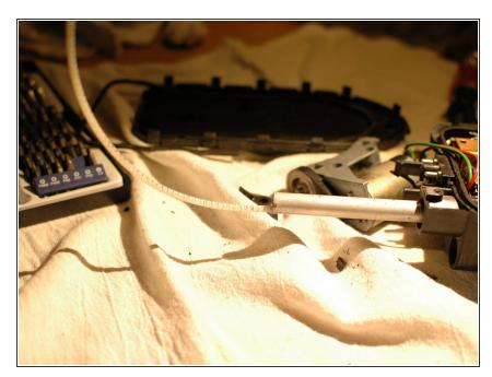
Pull the ribbed plastic cable connected to the antenna shaft out of the body of the motor.
