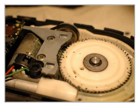
You can see the accumulation of dirt and debris on these gears. If the antenna shaft had not seized it would only have been a matter of time before the gears wore or broke.
