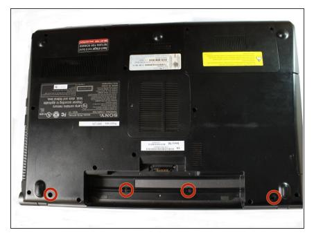
Remove the screws and flip it back.
