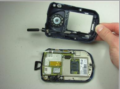
Pry open back plate using spudger.
