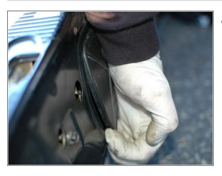
Remove this black plastic cover by prying it up from the bottom until it pops out enough to remove fully.
