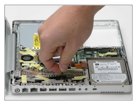
Use the black plastic pull tab to disconnect the display data cable from the logic board.
