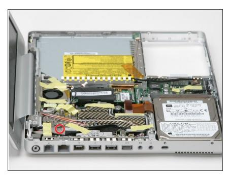
• Remove the Phillips screw securing the display data cable to the metal framework.
