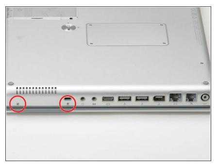
• Turn the computer 90 degrees clockwise and remove the two medium-length Phillips screws from the casing.
