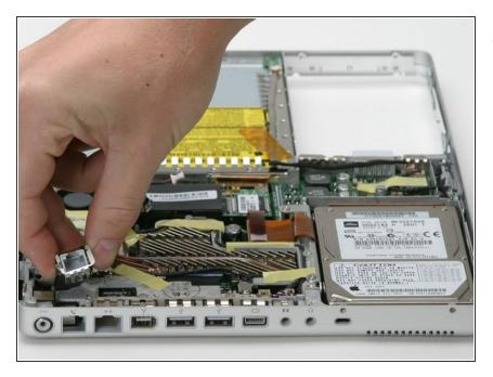
Lift up on the left side of the RJ-11 Board and remove it from the computer.
