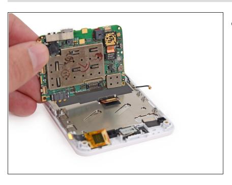
Remove the motherboard from the display assembly.
