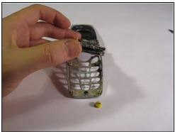
• Using your fingers or the pointed end of a black plastic spudger, pry the microphone out and replace.
