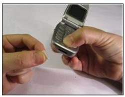
• The phone may have a rubber insert in the bottom of the phone (see picture). If this rubber insert exists, remove it from the bottom of phone and set aside.
