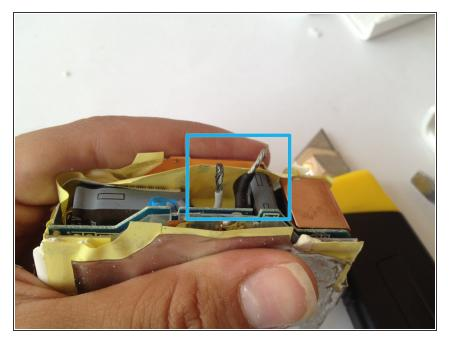
• Peel the plastic off the cable with a knife or a wire stripper.
