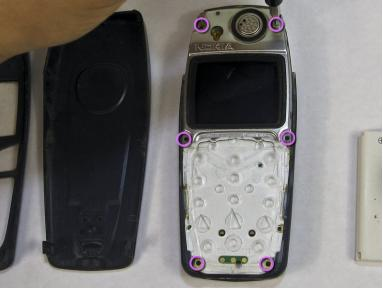
Remove the six screws around the front of the phone body with a T6 screwdriver.
