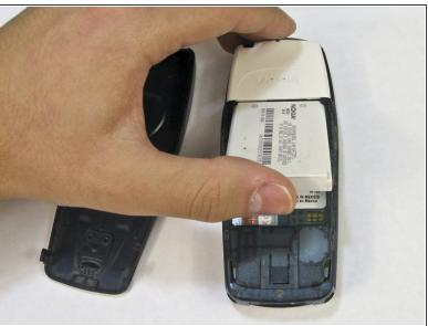
Lift the battery near the bottom and pry up.
