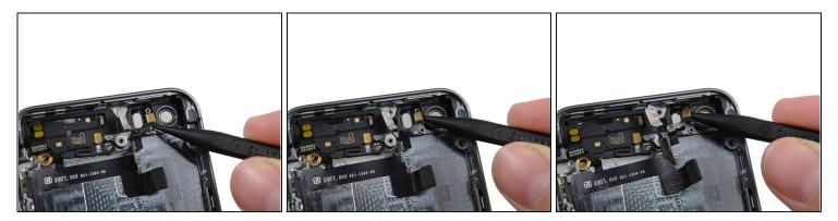
• Use the tip of a spudger to free the microphone portion of the assembly from the case.
