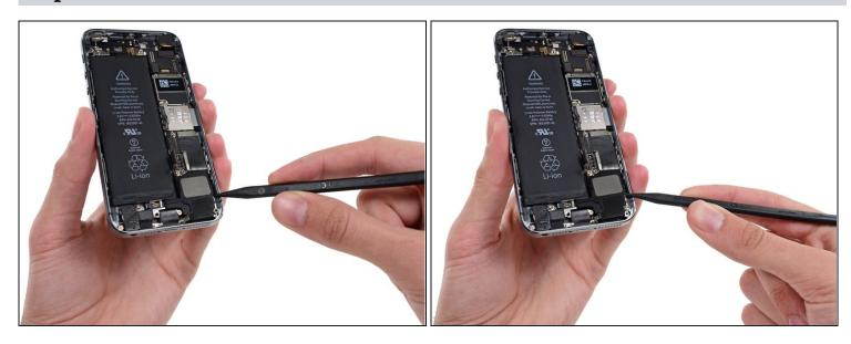
• Use the point of a spudger to gently pry between the speaker and the rear case, lifting the speaker enough to grab with your fingers.
