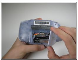
Take the battery cover off by releasing the locking tab and hinging the cover away. Remove the batteries inside the cover
