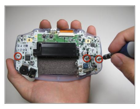
Remove the three screws on the circuit board with a Phillips #1 screw driver.
