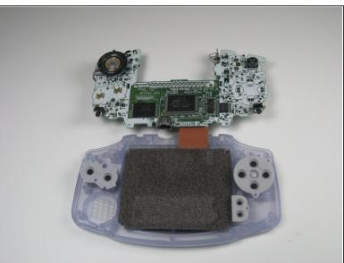
Pull circuit board away from the front panel by pulling up at the bottom of the circuit board, keeping the top ribbon still connected.
