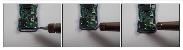
(i) There may be some solder in the way of the USB jack's metal contacts. If this occurs simply melt the solder to create room for the contacts.
