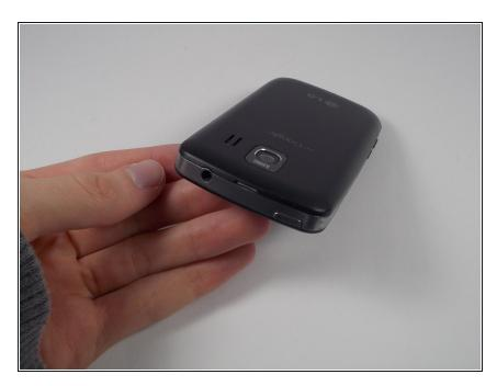
Turn the LG Optimus V over, so that the back cover is facing upward.
