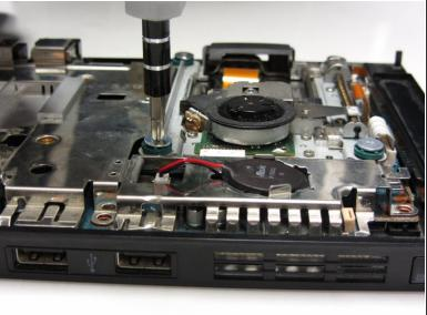
Remove the four 4.0 mm screws using a #1 Phillips screwdriver.
