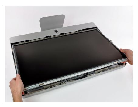
Disassemble iMac LCD panel according to existing guide iMac Intel Repair
