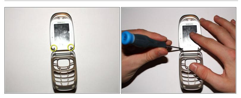
Remove the two highlited screws from the phone below the screen in order to open the display area.
