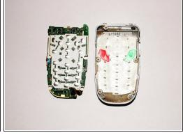
Remove the logic board from the phone by gently lifting up on the large green logic board with the plastic opening tool.
