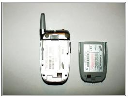
Slide the grey tab foreward and pry the battery up and out of the phone.
