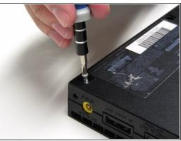
Remove all six 4.0 mm screws from the base of the unit using a #1 Phillips screwdriver.
