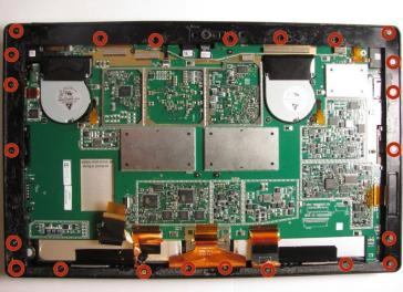
• Unscrew all the 23 screws located on the outside panel with the T5 torx screw driver
