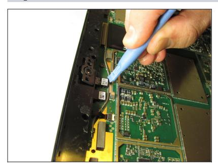
Use the plastic opening tool to pry out the cameras
