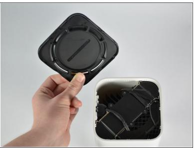
Using a metal spudger, gently pry the cover off the bottom of the device.
