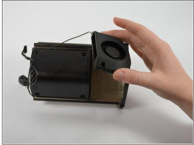
Remove the fan from the device.
