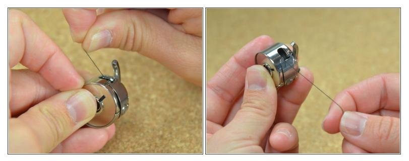
Slide the thread from the slit straight up along the groove and into the open hole on the bobbin case's side.
