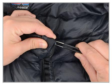
• Carefully remove any remaining pieces of the stop using tweezers.
