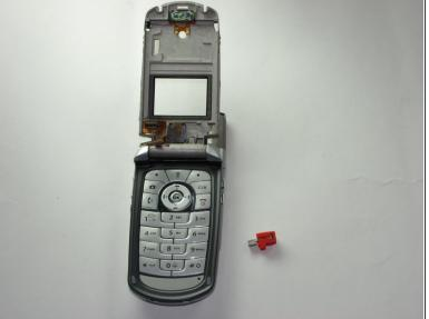
• Remove the vibrating motor from the phone with the spudger.
