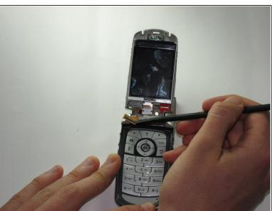
Use the spudger to pry upward and remove the plug that connects the screen to the main body of the phone.
