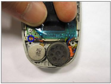
$\triangle$  Try not to move the thin component wires as they will bend and break very easily.
