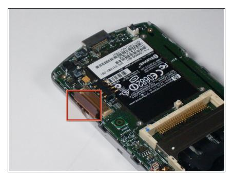
Carefully remove the orange LCD strip from the connector.
