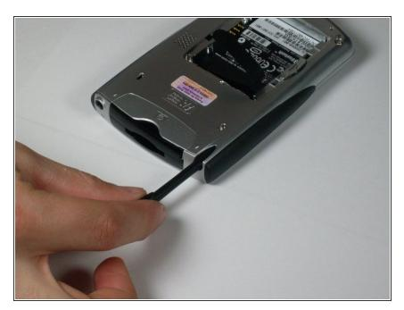
Remove the stylus by sliding it out of the slot.
