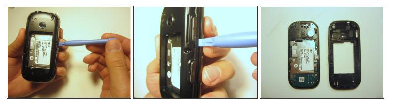
• Use the plastic opener to pry the rear case loose.
