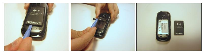
• Use the plastic opener to lift, and remove, the device battery.
