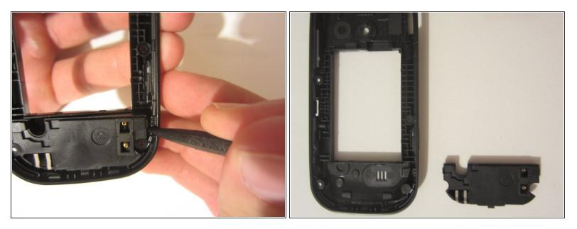
Use the TOOL to pry open the plastic piece located at the bottom of the rear case. This piece contains the speaker.
