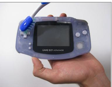
• Use a slightly damp toothbrush to scrape in between the desired sticky buttons. You can also use a bit of isopropyl alcohol.
