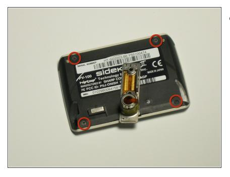
Remove 4 screws from back of screen.
