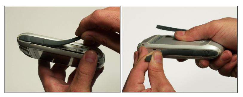
• The bumpers on the top and bottom of the phone can be removed by simply "peeling" them off.
