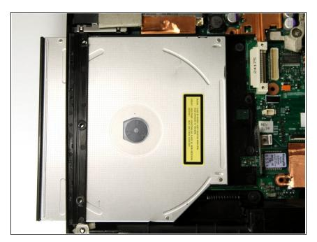
Slide the optical drive out of the laptop through the opening on the left side of the bottom assembly.
