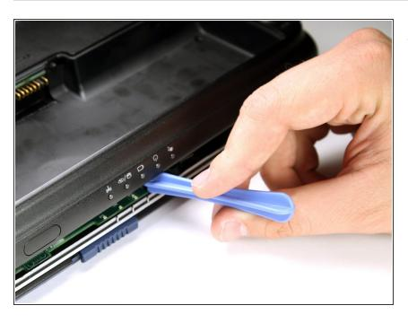
Use the plastic opening tool to pry the two halves apart.
