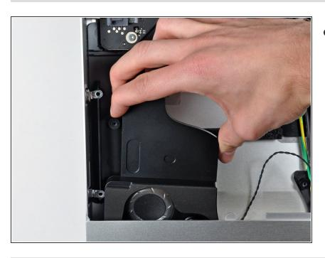
Lift the left fan toward the center of the iMac and remove it from the outer case, minding any cables that may get caught.
