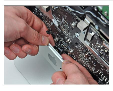
Use your fingers to lift IR sensor assembly straight up out of the outer case.
