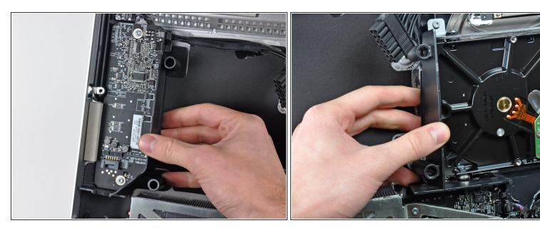
Remove the plastic ducts from the side of the LED driver board and the hard drive by pulling them away from the outer case.
