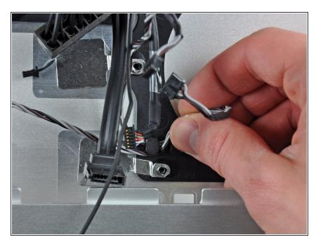
De-route the left speaker cable from the clips securing it to the outer case.
