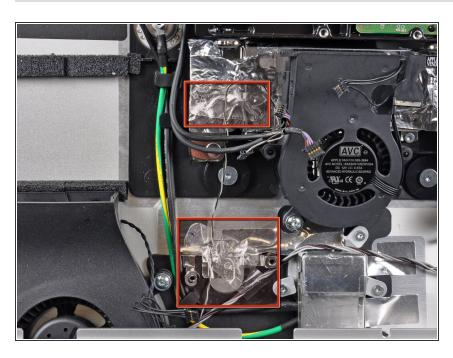
If present, remove the pieces of clear tape securing the ambient temperature sensor cable and the left speaker cable to the rear case.
