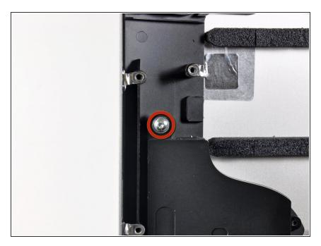
Remove the single 13 mm T10 Torx screw securing the left fan to the outer case.
