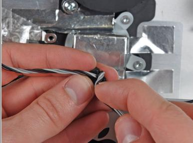
Carefully remove the left speaker and ambient temperature sensor cables from the CPU fan cable retainer.
