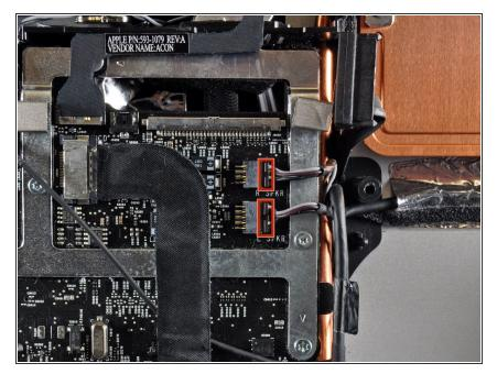
Pull the left and right speaker connectors toward the right side of the iMac to disconnect them from the logic board.
