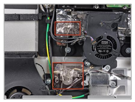
If present, remove the pieces of clear tape securing the ambient temperature sensor cable and the left speaker cable to the rear case.
