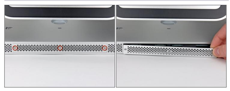
Loosen the three Phillips screws securing the access door to the bottom edge of your iMac.
