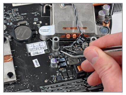
• Use a pair of <u>tweezers</u> to lift the heat sink thermal sensor connector straight up out of its socket on the logic board.
