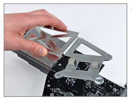
• Lift the heat sink bracket off the logic board.
