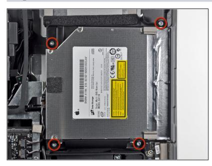
• Remove the four 9 mm T10 Torx screws securing the optical drive to the outer case.
