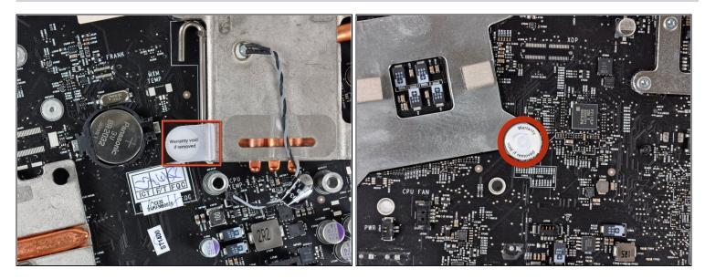
(i) If present, remove the "Warranty void if removed" stickers covering one screw on either side of the heat sink.
