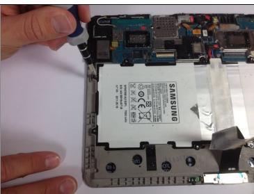
Remove the ten 3 mm Phillips #00 screws surrounding the battery.
